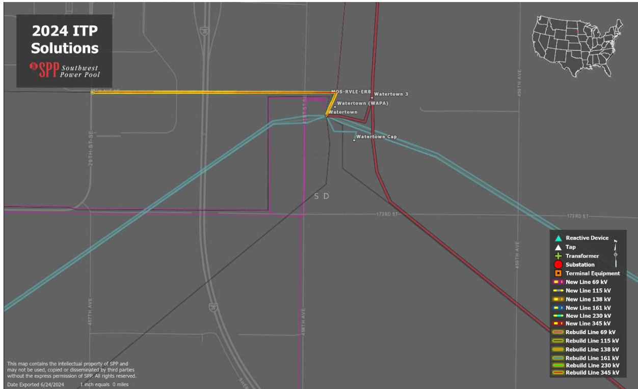
Figure 6.41: UMZ: 15th Ave – Watertown 115 kV Rebuild
